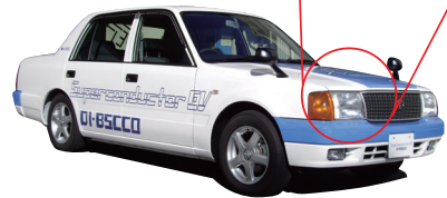
超電導電気自動車 (試作車) EV with superconducting motor (vehicle remodeled)
