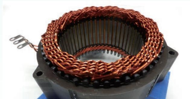
**12 Rectangular Magnet Wires for Electrified Vehicles**
