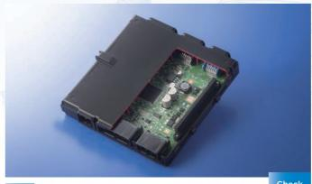
**Smart entry function integrated BCM** Sumitomo Wiring System
